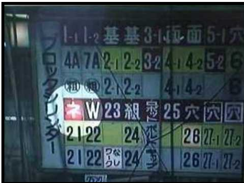
3. Probe signals an “andon” board for visual display
