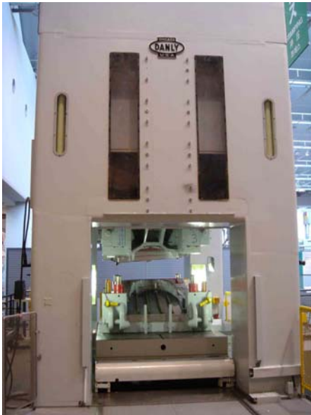
Same 1960 Danly press with moving bolster mechanism side view.
