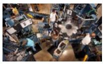
Utilizing the lean manufacturing system, assembly line stations on the floor at Dura Automotive are designed around the workers, funneling parts within reach to minimize movements and increase productivity.
